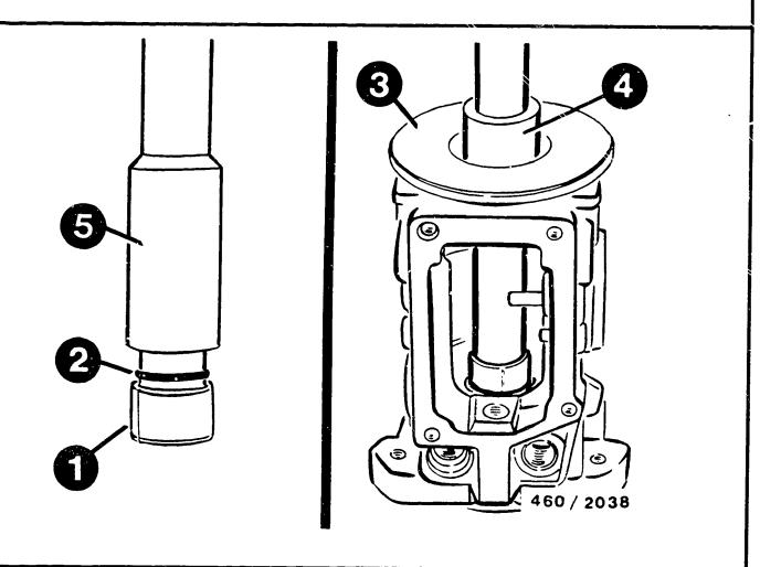
Insert holding fixture KDEP 1170/6 into pump housing. Position fuel—injection—pump housing with holding fixture on support plate of mandrel press.
